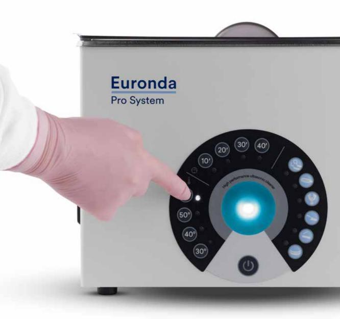
There are two operational modes, allowing users to choose one of the 6 preset cycles (instruments, burs, impression trays, cement removal, plaster removal, and prostheses) or run a free cycle at a temperature between 30°C and 60°C, with a duration between 10 and 40 minutes. There are 4 different operating stages in the 6 preset cycles: Degas, Boost, Normal and Sweep.
